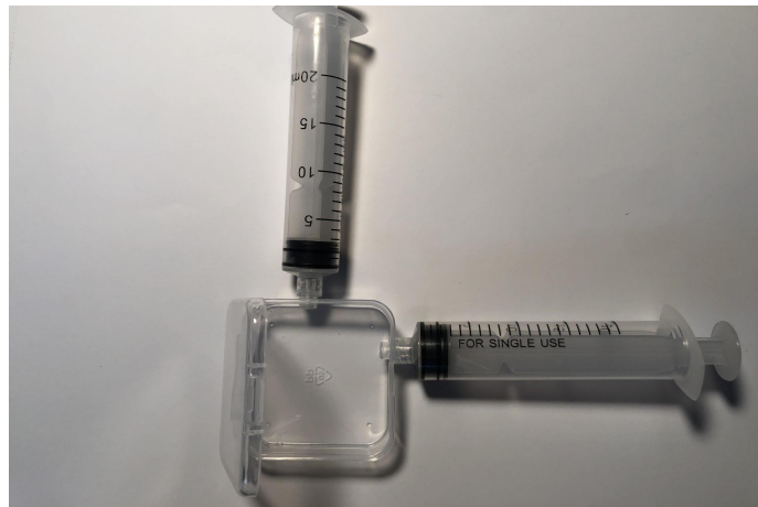
Fig. 9 - Plastic, hinge top box drilled to accept female Luers.
