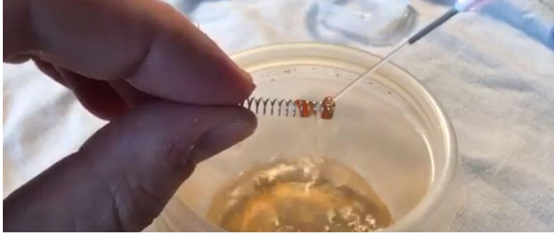
Fig. 3 - Base test with a 20mL syringe angled at 45° to the spring, squirting a jet of tap water at a ketchup clot.
