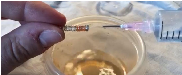
Fig. 4 - Base test with a 20mL syringe parallel to the spring, squirting a jet of tap water at a ketchup clot.
