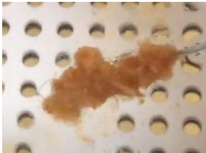
Fig. 7 - Ultrasonic cleaner dissolving some of the oils off of the jackfruit loaded stent retriever. This device was unable to detach the fibrous jackfruit from the tines.
