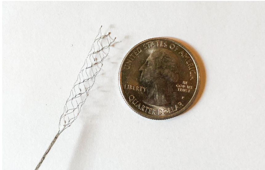
Fig. 5 - Medtronic Solitaire™ X stent retriever received from Dr. Rivet for testing purposes.
