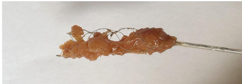
Fig. 6 - Jackfruit loaded stent retriever for testing in the small Ultrasonic cleaner.
