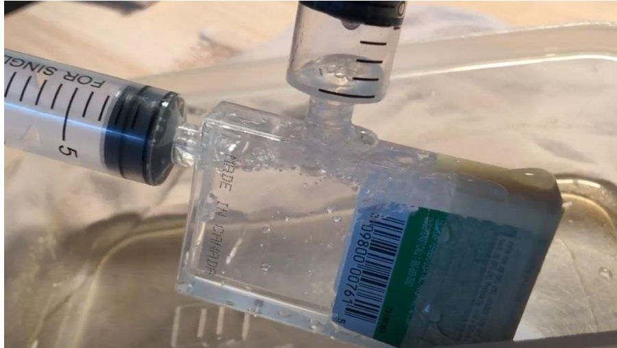
Fig. 10 - Agitated bubble chamber created from a Tic Tac® box. Note the water droplets still escaping around the top of the box where the tape is.
