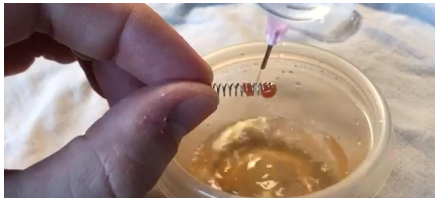
Fig. 2 - Base test with a 20mL syringe perpendicular to the spring, squirting a jet of tap water at a ketchup clot.
