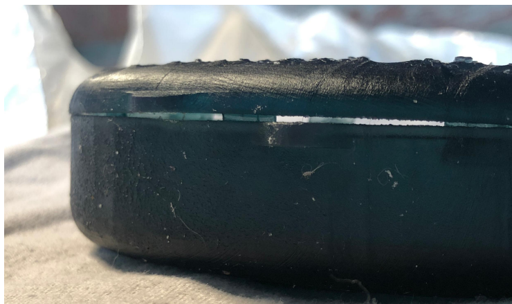
Fig. 36 - Early resin prototypes with visible gap between the top and bottom
